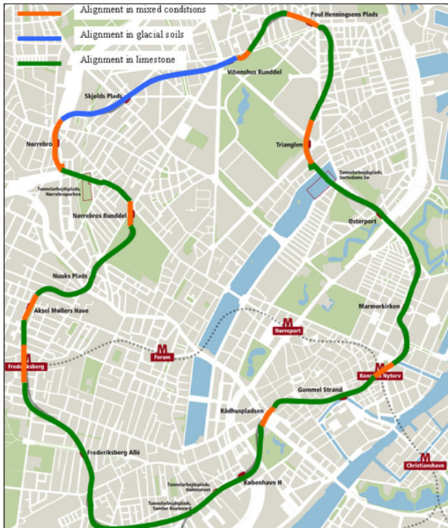
Figure 7. Ground conditions along the tunnel alignment
